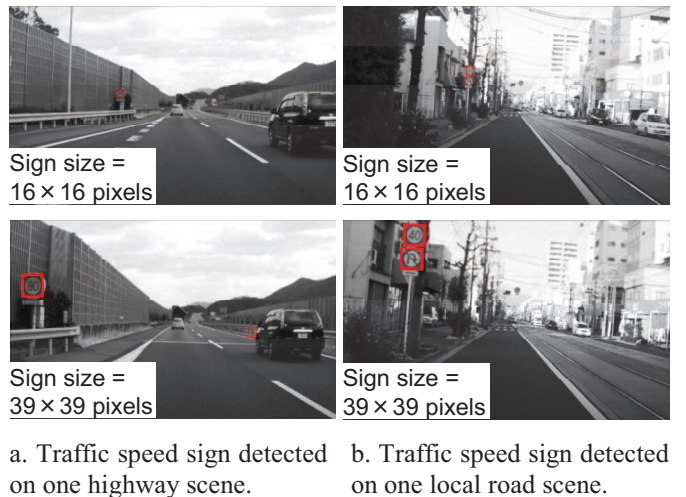
Fig. 2. Examples of ROIs detected in the real life in daily condition at different distances.
