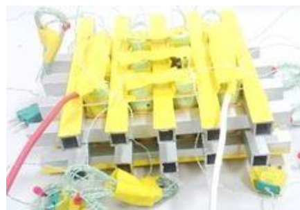
Fig.14. Cooling system for assembled battery
