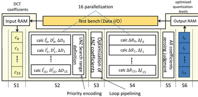
Fig. 1. Block diagram of RDOQ processing module
