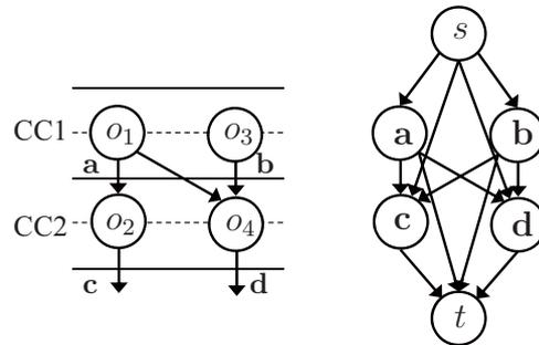
Fig. 4. Example DFG (left) and the corresponding graph for our heuristic algorithm (right).
