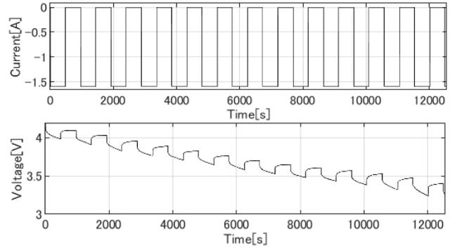
Fig. 5. The test discharge waveform pattern 1
