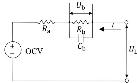
Fig. 2. The equivalent circuit model of the Li-ion battery
