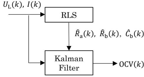
Fig. 3. Block diagram of OCV estimation using the joint method of Kalman filter and RLS
