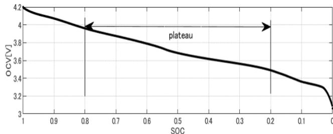
Fig1. OCV-SOC curve
