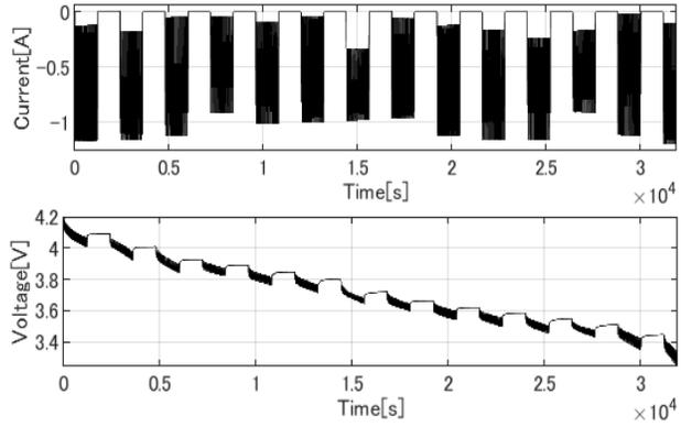
Fig. 7. The test discharge waveform pattern 1
