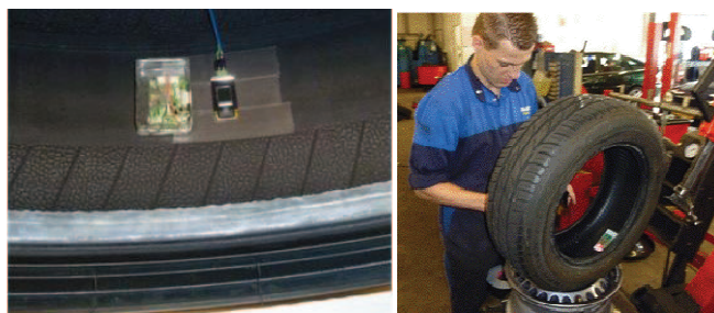
Figure 10: Left: Energy harvester and wireless sensor system for measurement of accelerations mounted in tire. Right: mounting of tire on rim in tire shop.
