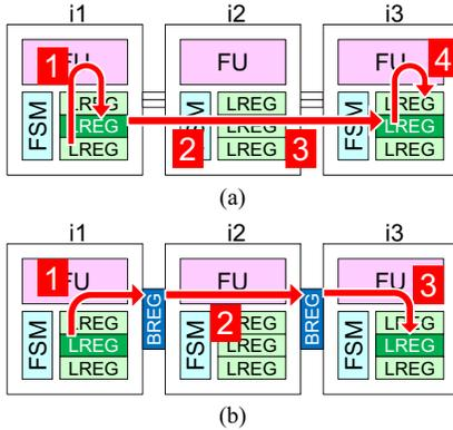
Fig. 2. Computations and data transfer. (a) In RDR architecture. (b) In RB architecture.
