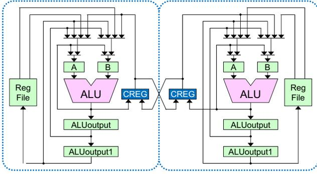
Fig. 8. Regular distributed register architecture.
