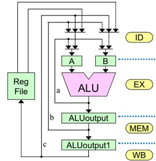
Fig. 4. The datapath of DLX processor.
