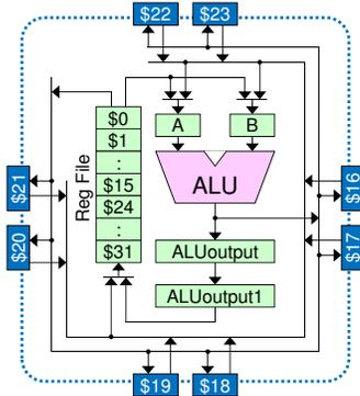
Fig. 6. The extended processor for RB architecture.
