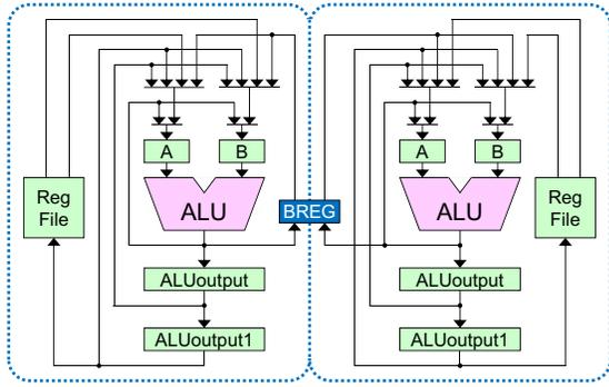
Fig. 5. Bridge-register architecture.
