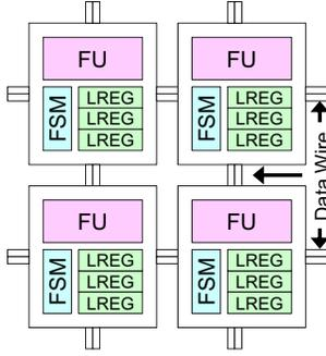
Fig. 1. Regular distributed register architecture.
