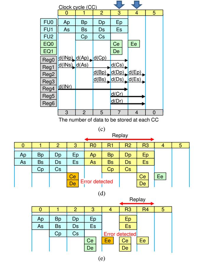
Fig. 2. Error-free input data for error correction by replay. (a) a DFG. (b) DMR schedule for operations and data. (c) error detection schedule and the necessary input for replay. (d) replay invoked when an error is detected at CC 3. (e) replay invoked when an error is detected at CC 4.
