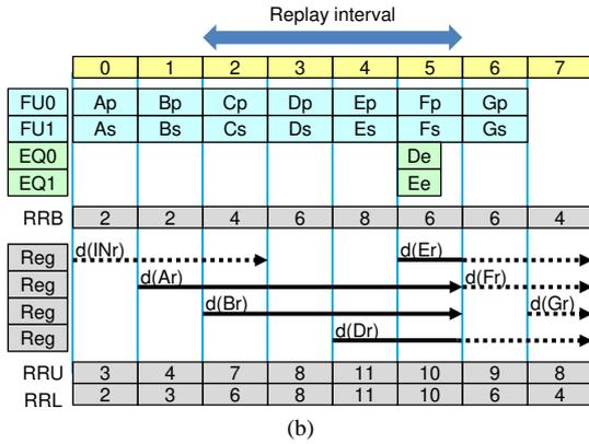
Fig. 4. The upper and lower bounds of register requirement. (a) for  $Replay(3, 6)$ . (b) for  $Replay(2, 5)$ .
