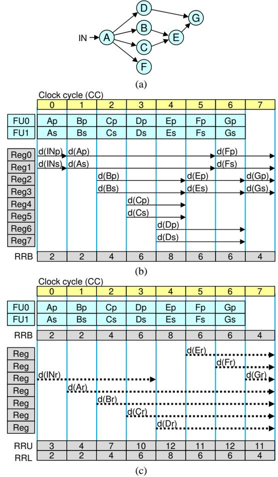
Fig. 3. Register requirement for DMR. (a) a DFG. (b) baseline register requirement for the primary and secondary operations. (c) the upper and lower bounds of register requirement when no replay interval is considered.
