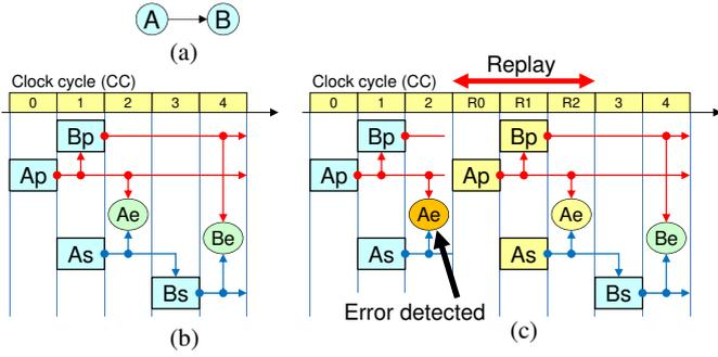
Fig. 1. An example for error correction by replay in DMR. (a) a DFG. (b) DMR schedule for operation execution. (c) replaying the schedule when an error is detected.
