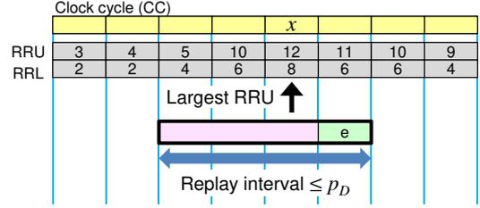
Fig. 5. Replay interval including the CC with the largest RRU.
