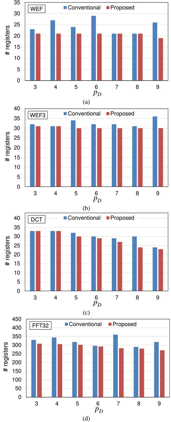
Fig. 7. The result of the register minimization. (a) WEF, (b) WEF3, and (c) DCT with 6 adders and 6 multipliers. (d) FFT32 with 40 adders and 40 multipliers.
