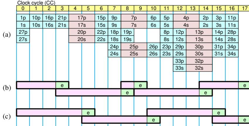
Fig. 8. The resultant set of replay intervals. (a) a DMR schedule for WEF with 6 adders and 6 multipliers. (b) the result obtained by the proposed method. (c) the result obtained by the conventional method.
