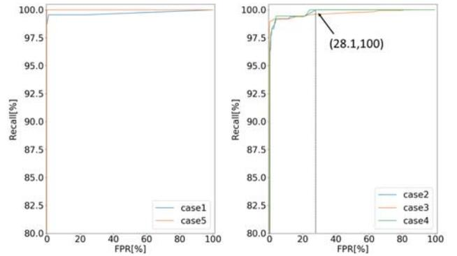
Fig. 8. ROC curve in case1 to case5. Recall and FPR are in the relationship of trade-off. The closer the curve is to the upper left, the better result it shows. In case2, if you lower the threshold until 100 % Recall is achieved, FPR will increase to 28 %.
