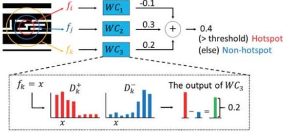
Fig. 4. The configuration of the hotspot detector is shown. In this example, the detector consists of three weak classifiers corresponding to the determined circles. The output of each weak classifier is determined according to the difference between the probability of the feature value derived from hotspot clips and that from non-hotspot clips. If the sum of outputs exceeds the threshold, an input clip is regarded as hotspot.
