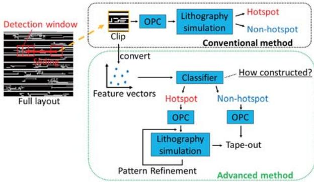
Fig. 1. Comparison of conventional and recent advanced methods. In advanced methods, a number of clips are filtered out in advance by classifiers, and the number of lithography simulations required is reduced.
