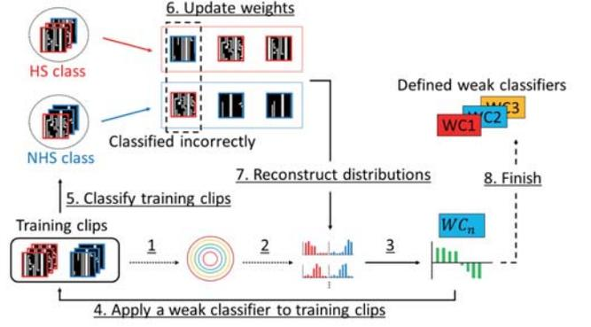
Fig. 5. The flow of training the detector is shown. The probability distributions can be easily computed using training data (flow.1-2). A weak classifier is defined based on feature optimization using them (flow.3). It's applied to training clips and classifies them (flow.4-5). By increasing the weights of clips classified incorrectly, distributions are reconstructed (flow.6-7). Flow.3-7 are repeated to define multiple weak classifiers.
