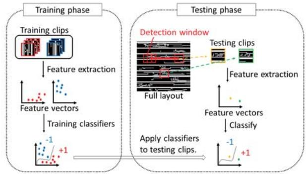
Fig. 2. The basic idea of machine learning based hotspot detection. Using known hotspot/non-hotspot clips given as training dataset, the classifier is trained. It is applied to testing clips extracted from a mask, and judge whether each clip is hotspot or not.
