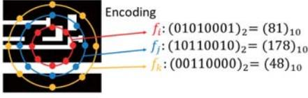
Fig. 3. The process of calculating layout features using CCAS. Each sampling circle is encoded to compact representation.
